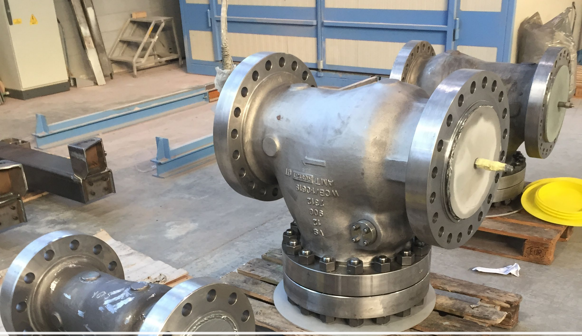
SWING CHECK VALVE Preparation for painting process.
