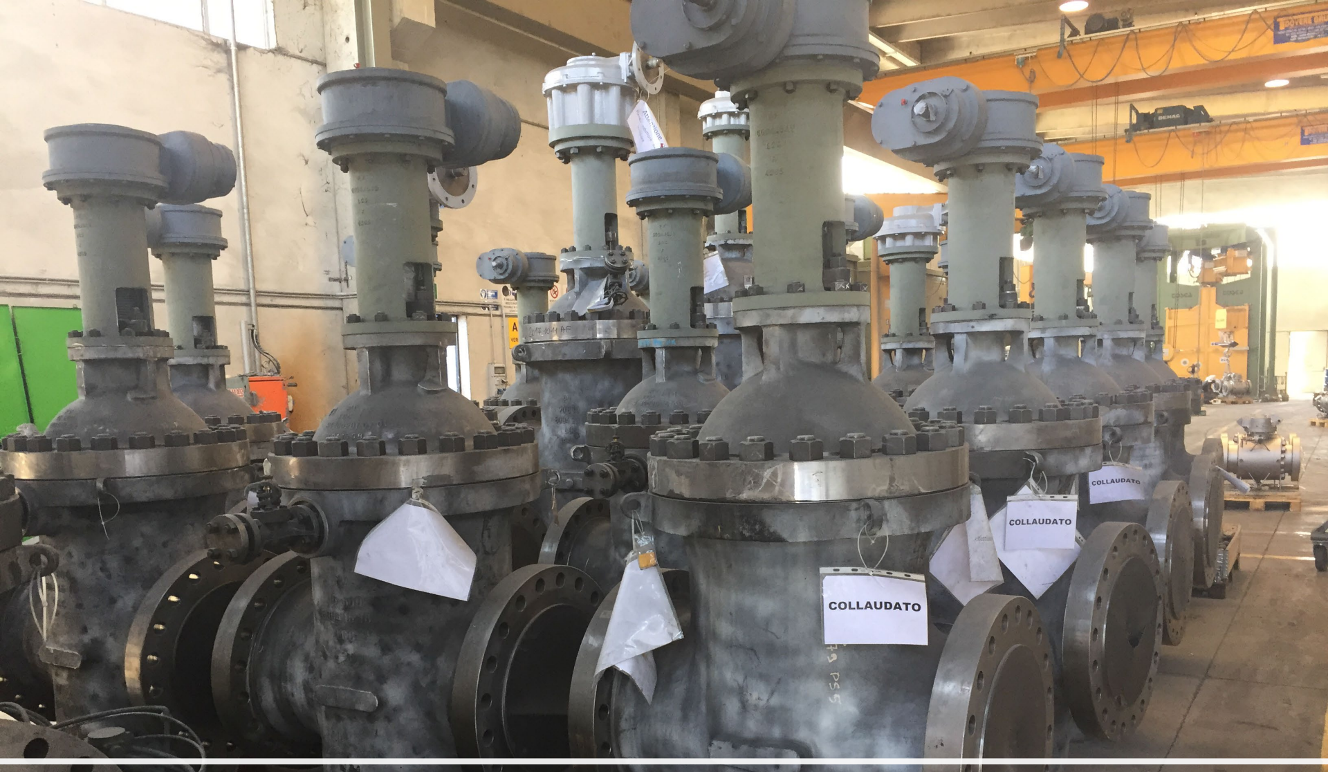
THROUGH CONDUIT GATE VALVE Ready for painting process.
