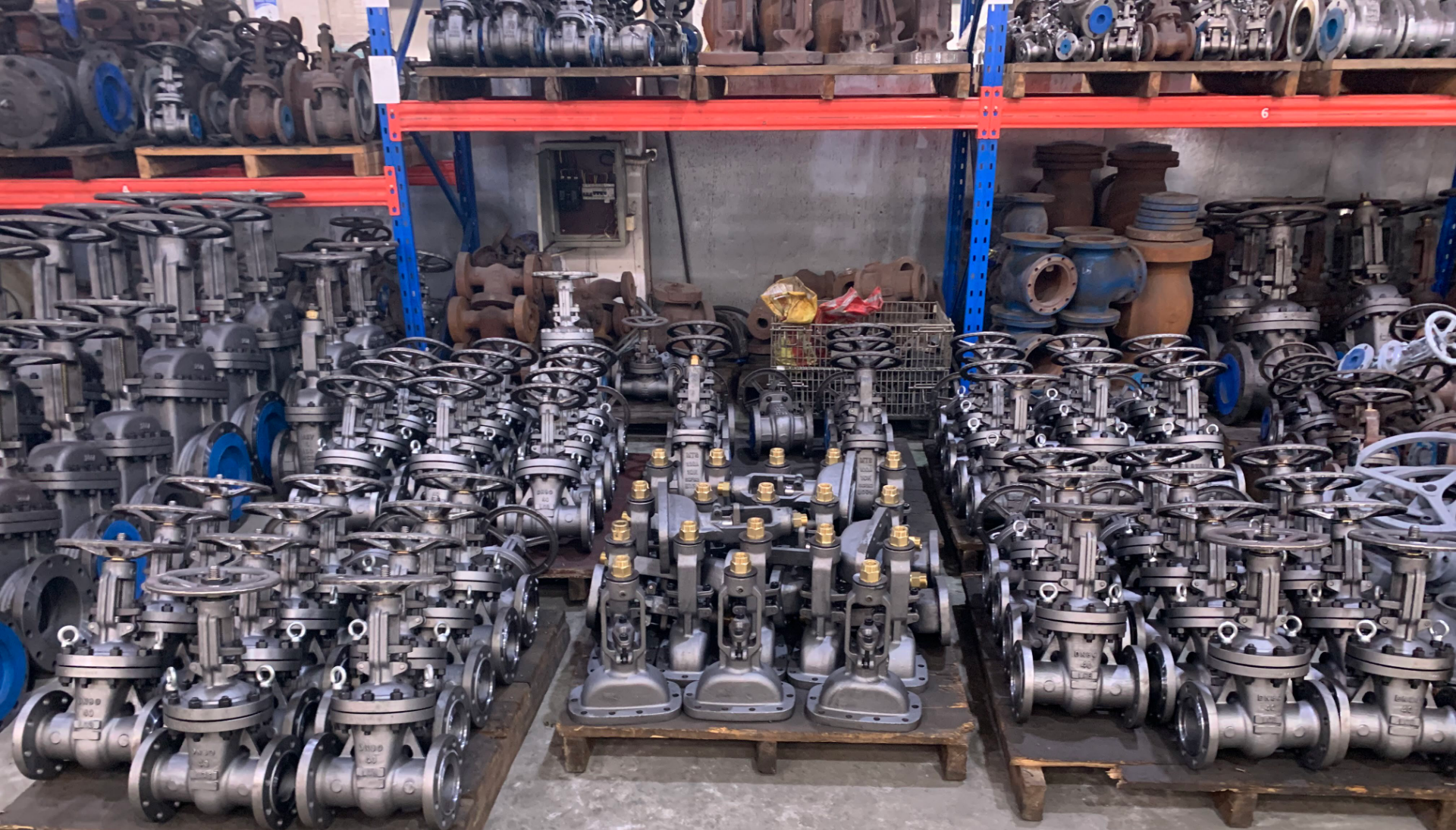
MANUAL GATE VALVES Under Assembling.
